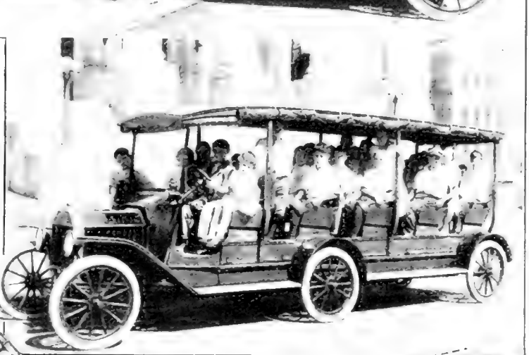
Above: An ingenious six-wheeled automobile, with the body mounted flexibly on the frame at two points (Autoport System)
